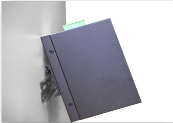
Figure 3.2 - Insert the Switch on the DIN-Rail
